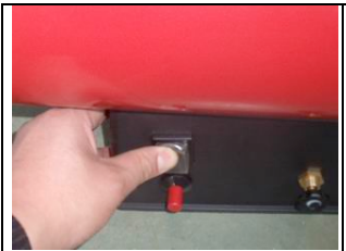
put the power switch at position "1"
