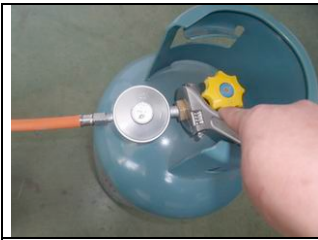
Tighten the connector according to the arrowhead direction
